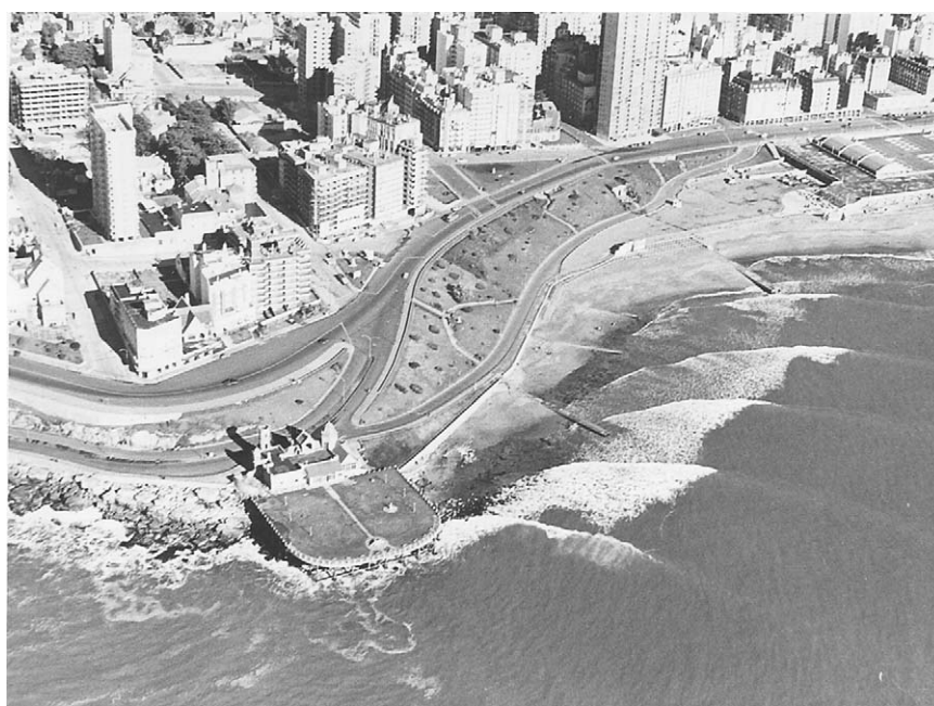
Fig. 3. Air view (1980s) of the central beaches of Mar del Plata close to a rocky headland (very hard quartzite) showing the defense works and the pattern of sediment transport to the right (northward).
