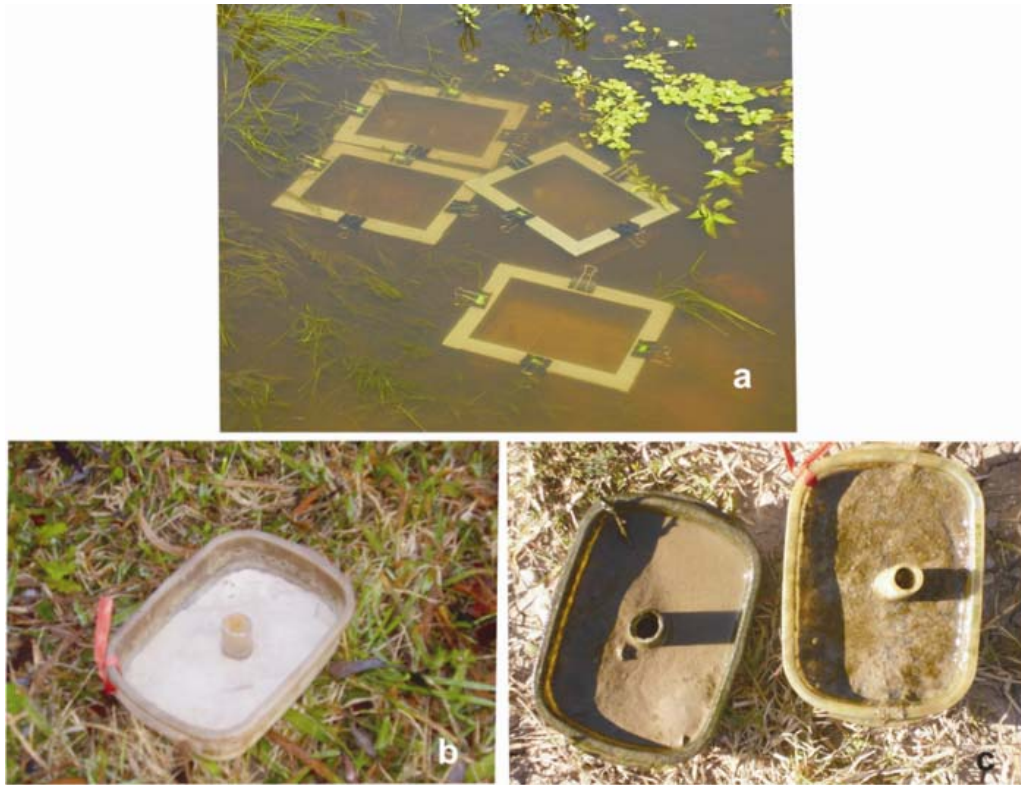
Figure 8. a) Metabolism chambers employed to measure metabolic variables, b) Artificial substrata used for biofilm attachment, c) Artificial substrata after the 4-week period necessary for colonization of the biofilm
