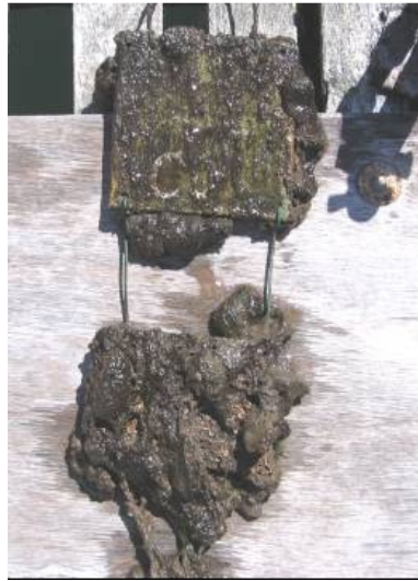
Photograph No. 2: General aspect of panels with Amercoat 235 + Cu covering (upper panel). Control panel (lower panel). 365 days of immersion.
