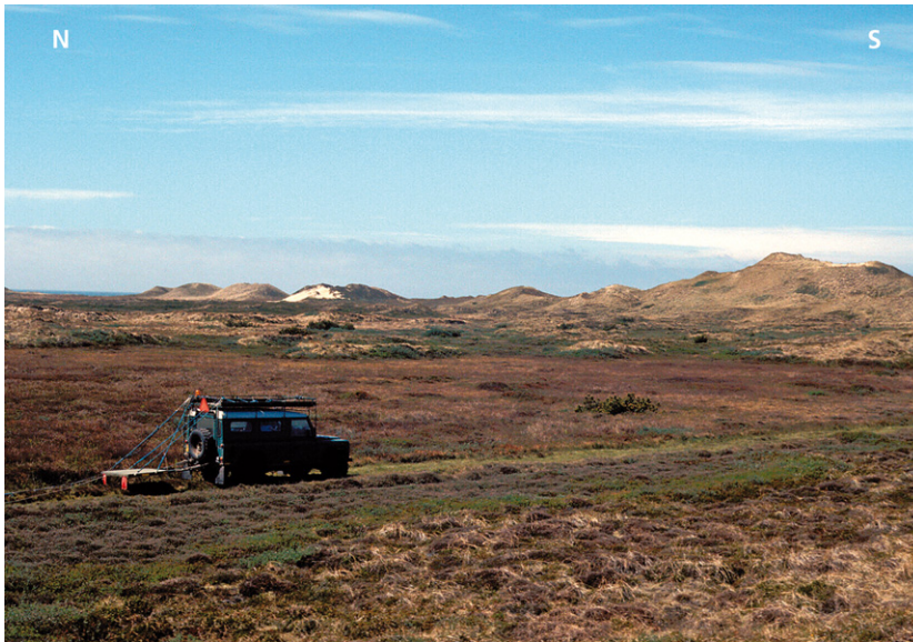
Fig. 14. Ground-penetrating radar mapping of sedimentary architecture; coastal dune field at Lodbjerg, Denmark (Clemmensen et al. , 2001a). The surface of the modern dune field is situated ca 15 m above sea-level, and the dune field is truncated by a coastal cliff towards the North Sea. Partly active cliff-top dunes are developed along the cliff. Vehicle for scale is ca 5 m long.
